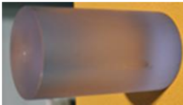
Fig. 11 Shape of projectile used in penetration test
